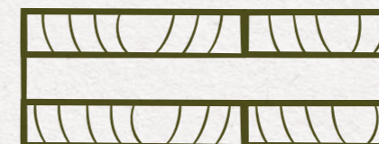
Basic structure of 3-layer-cross-laminated timber
